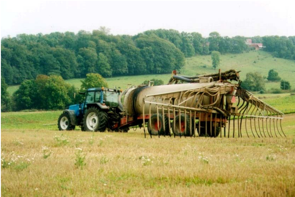
Figure 4.2.1 Hose spreader for spreading liquid manure, Helsingborg
